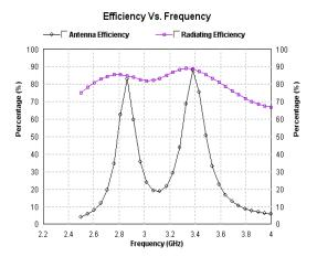
**Fig: 5.** Radiation & antenna efficiency graph Also figure number 6 shows the radiation pattern of an antenna.
